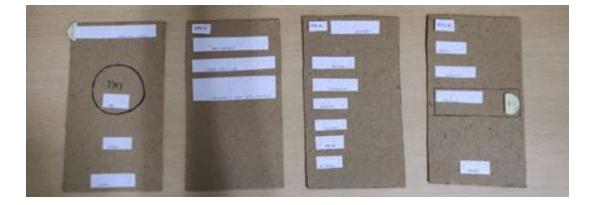
As our target audience is visually impaired, we made Braille tag for the functional button to ensure readability. We made a low fidelity prototype of the screen out of cardboard instead of paper to ensure stiffness since the user would be pressing against the braille tags to interpret the text.
